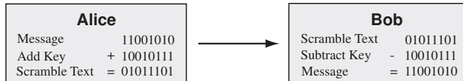
Figure 3.2: The One-Time Pad is the only known classical cryptography protocol that is completely secure. Here the key is added by Alice and subtracted by Bob, using modulus 2.
